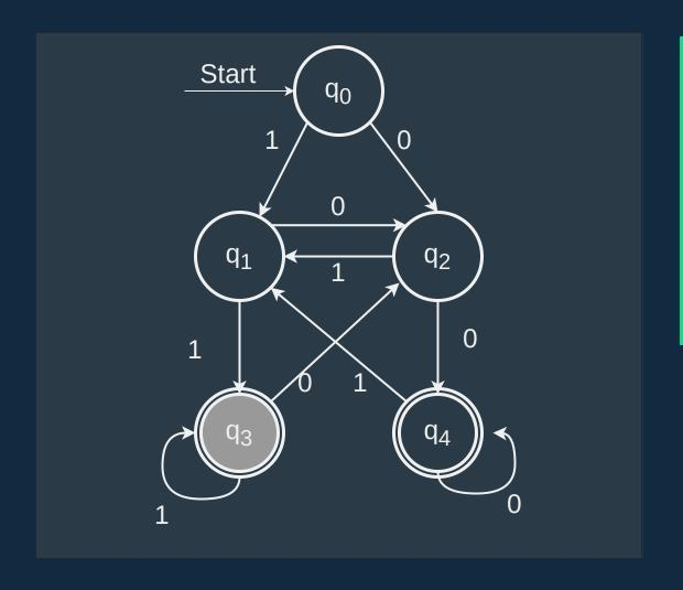
No matter where we start in the automaton, after seeing two 1's, we end up in accepting state  $q_3$
