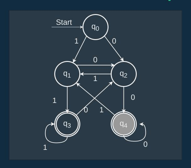
No matter where we start in the automaton, after seeing two 0's, we end up in accepting state  $q_4$
