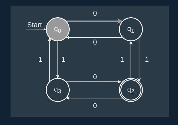
Each arrow in this diagram represents a transition. The automation always follows the transition corresponding to the current symbol being read
